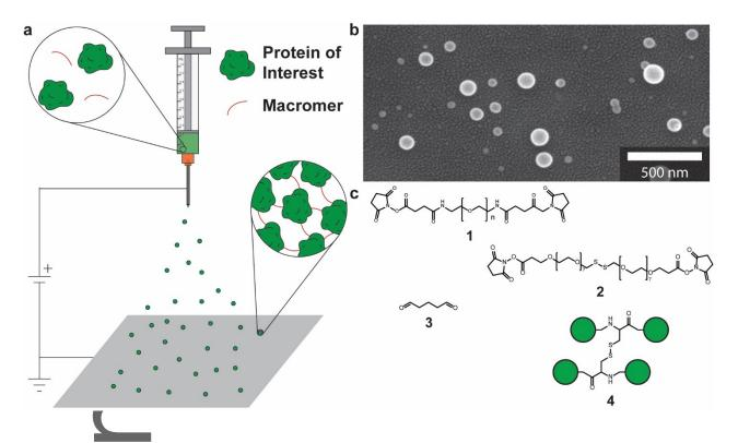
**Figure 1.** (a) Preparation of Synthetic Protein Nanoparticles (SPNPs) using reactive electrojetting. (b) SEM images of particles made using EHD jetting. Particles are jetted, and subsequently (c)polymerized using a variety of different macromers: 1. (PEG-NHS), 2. (PEG-NHS-S), 3. (GA) and 4. (S-S)
