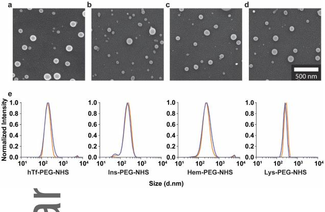
**Figure 2.** Stable synthetic PNPs can be made using a variety of proteins. SEM images of SPNPs made from (a) hTf-PEG-NHS, (b) Ins-PEG-NHS, (c) Hem-PEG-NHS, and (d) Lys-PEG-NHS. (e) The stability of particles in PBS over a 1 week period was characterized by measuring the particles using DLS 1 day (blue trace) and 7 days (red trace) after synthesis and size purification.
