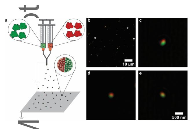
**Figure 4.** EHD co-jetting can be used to make bicompartmental SPNPs. (a) SPNPs containing Human Serum Albumin (HSA) in one compartment and Human Serum Transferrin (hTf) in the other were synthesized, with each compartment doped with BSA-Alexa-488 or hTf-Alexa-647, respectively. The particles were imaged using SIM. (b) The images were then deconvoluted. (c-e) Zoomed in images of individual particles are shown to showcase the bicompartmental nature of the particles.
