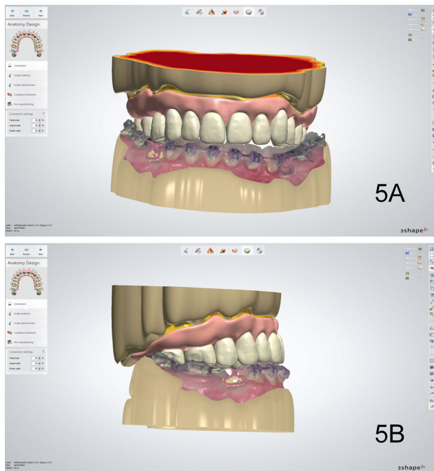
Figure 5 Virtual design of complete denture base and teeth: (A) frontal view; (B) lateral view.
