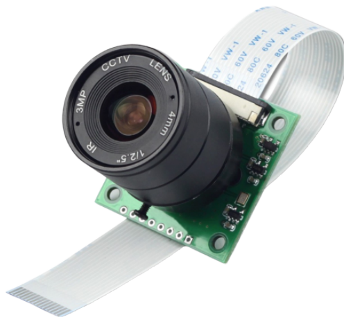
Figure 8: Arducam with Sony IMX219 and LS2718 lens
