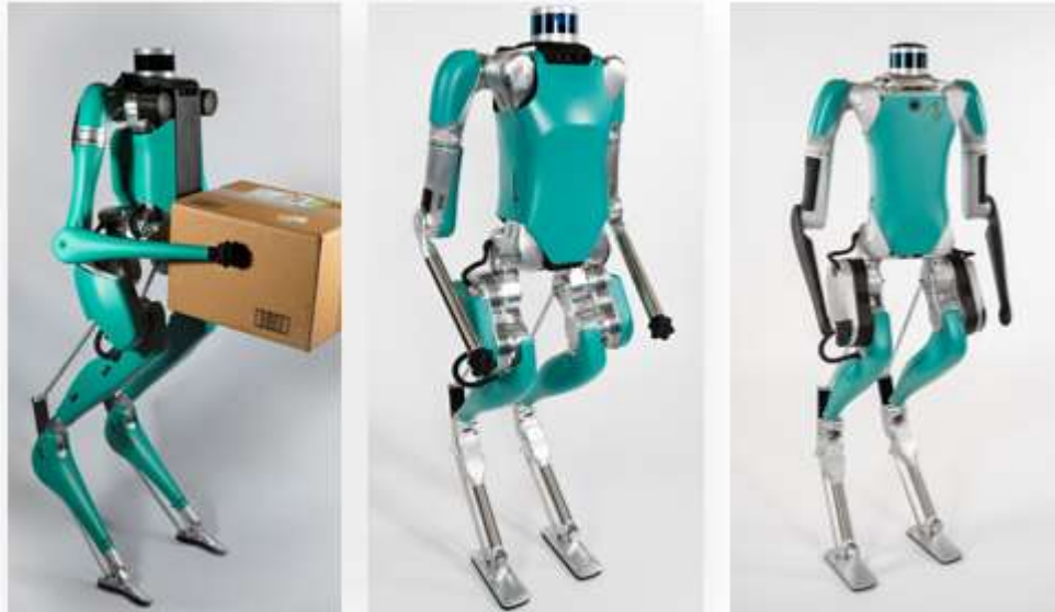
Figure S2. Agility Robotics Digit models, v1 (left), v2 (center), v3 (right). [Reproduced with permission from Agility Robotics]
