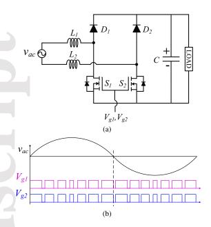
**Fig. 1**. (a) Classical bridgeless boost PFC converter. (b) Gating signals of switches.
