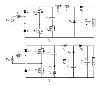
**Fig. 6**. (a) Hybrid resonant PWM bridgeless boost PFC converter. (b) Soft switching based bridgeless boost PFC converter.
