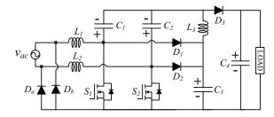
Fig. 12. Bridgeless SEPIC PFC converter with extended gain.
