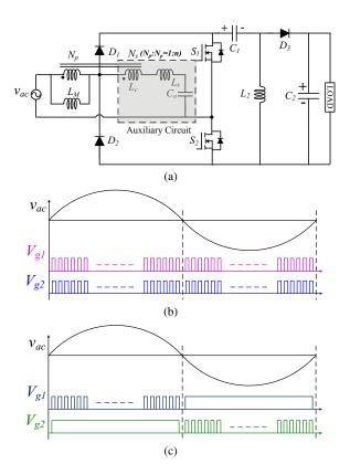
**Fig. 14.** (a) Bridgeless SEPIC converter with a ripple-free input current (b) Conventional gating signals for switches in bridgeless SEPIC converter. (c) The gating signals used for bridgeless SEPIC converter of Figure 14(a).
