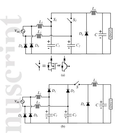
**Fig. 7**. (a) Bridgeless buck PFC converter with discontinuous capacitor Voltage mode (DCVM) using two switches. (b) Bridgeless buck PFC converter with discontinuous capacitor Voltage mode (DCVM) using single switch.
