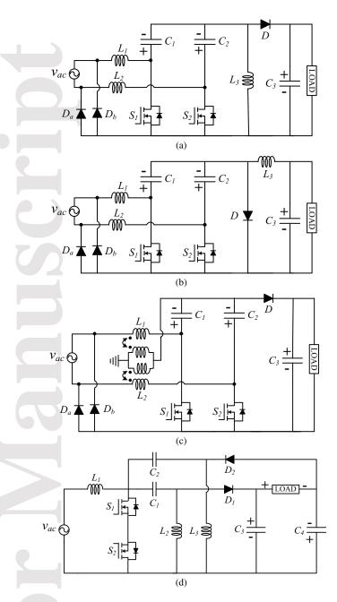
**Fig. 11**. (a) Bridgeless SEPIC PFC converter. (b) Bridgeless CuK PFC converter. (c) Coupled inductors based bridgeless SEPIC PFC converter. (d) A modified bridgeless SEPIC PFC converter.
