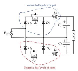
**Fig. 8**. Bridgeless buck PFC converter with voltage doubler output using two inductors.
