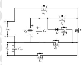
Fig. 15. A bridgeless based integrated converter for PEVs.
