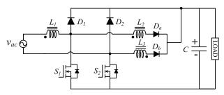
Fig. 5. Ripple free bridgeless boost PFC converter.
