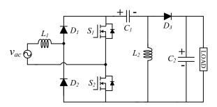
Fig. 13. Bridgeless SEPIC PFC converter with reduced components.
