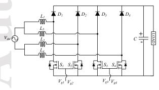
Fig. 4. Bridgeless interleaved boost PFC converter.
