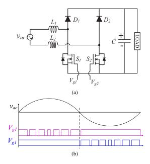
**Fig. 2**. (a) Phase shifted bridgeless boost PFC converter. (b) Gating signals of switches.
