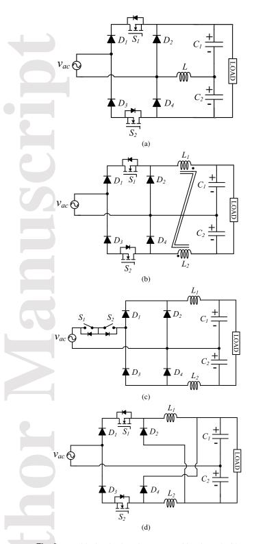
**Fig. 9**. (a) Bridgeless buck PFC converter with voltage doubler output using two inductors. (b) Bridgeless buck PFC converter with voltage doubler output using coupled inductors. (c) Bridgeless buck PFC converter with voltage doubler output using two inductors and two bidirectional switches. (d) Bridgeless buck PFC converter with nonlinear output using two inductors.
