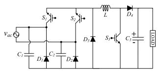
**Fig. 10**. Bridgeless buck/boost PFC derived from the cascaded buck/boost converter.
