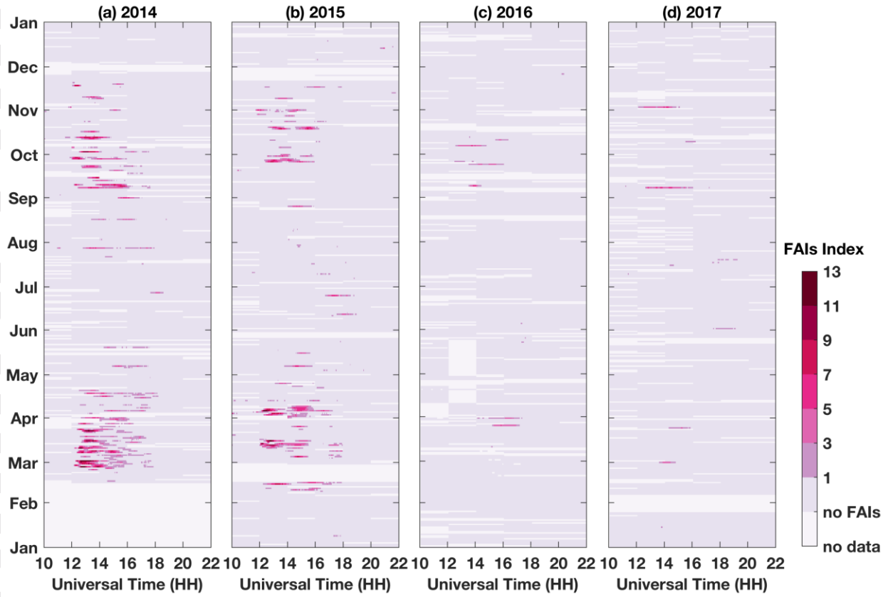
Figure 3. (a-d) Universal time and seasonal variations in the FAIs index (see text for explanation) observed by the HCOPAR from 2014 to 2017. FAIs index \geq 1 was regarded as echoes from FAIs.
