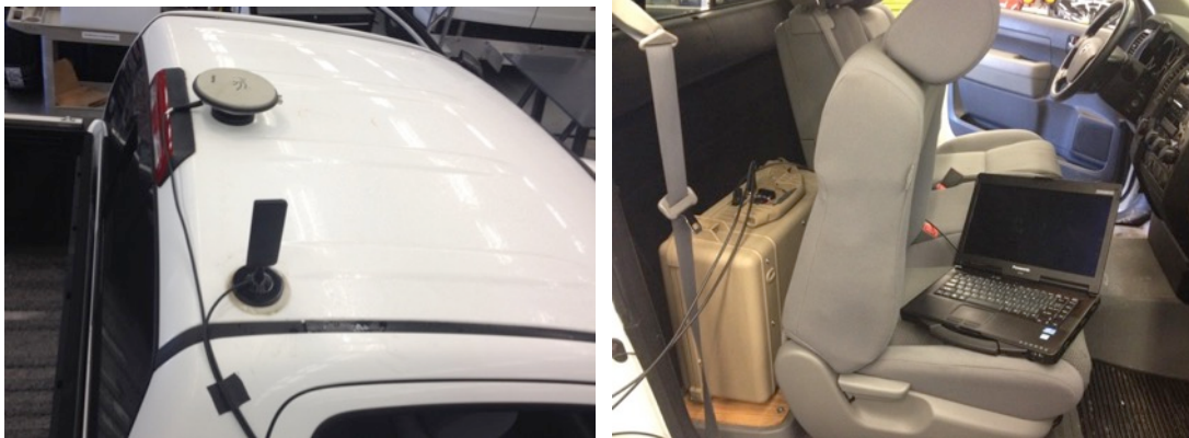
Figure 3.2 GPS system set-up
