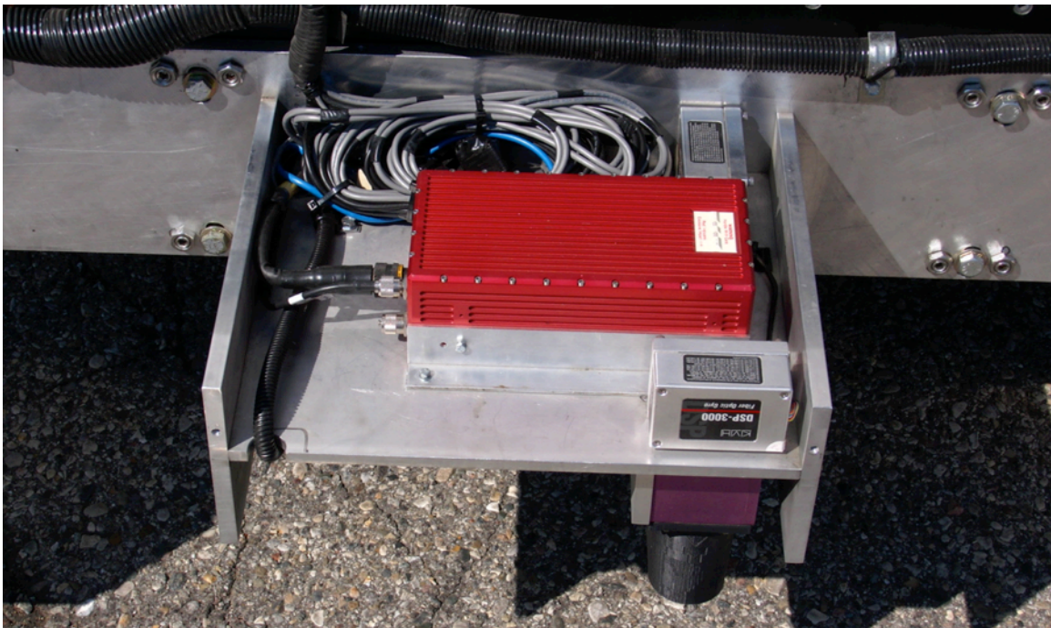
Figure B.8 Center sensor pod, cover removed
