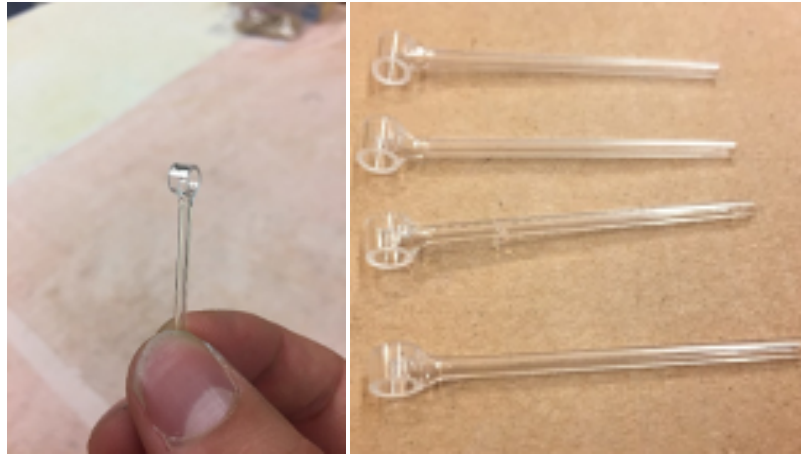
Figure 7.3: T-shaped glasses with filling stems. The longer, thinner stem is used as a Rb filling channel. The shorter, thicker cylindrical part attached on top of the filling stem is used for anodic bonding to silicon parts. These two parts are attached to each other using traditional glass-blowing techniques.
