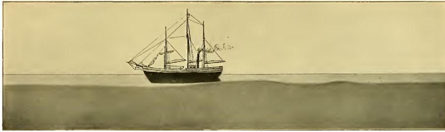
Fig. 1 To understand the “dead-water” phenomena, Ekman performed a series of experiments in a tank filled with fresh surface and ink-dyed salty bottom water layers. Ekman pulled a boat model, attached to a rope, with a constant force through the upper layer. This photograph shows the side of the tank, the Fram boat model, completed by a sketch of the upper part of the Fram, and internal waves on the layer interface behind the ship. Reproduced with permission from: Ekman, V. W. (1904). On dead water. In: Nansen, F. (Ed.), The Norwegian north polar expedition 1893–1896. Scientific Results , Vol. V. pp. 83–278. Christiania.
