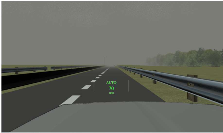
Figure 3.2: Driving task: to drive a vehicle on a highway and avoid the obstacles, with lane-keeping and alert assistance from the automated driving system.
