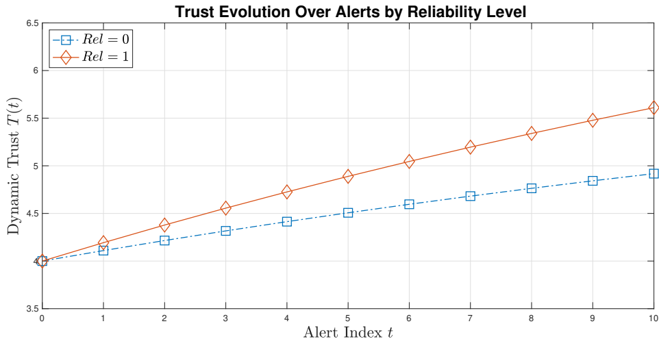
Figure 3.6: Curves illustrate the simulation of the model represented by Equation (3.5). We chose T(0) = 4 for both conditions to better compare the results. When Rel = 1 (i.e., when participants were using a reliable ADS), trust increased faster than when Rel = 0 (i.e., when participants were using an unreliable ADS). For both curves, Vis = 0 .
