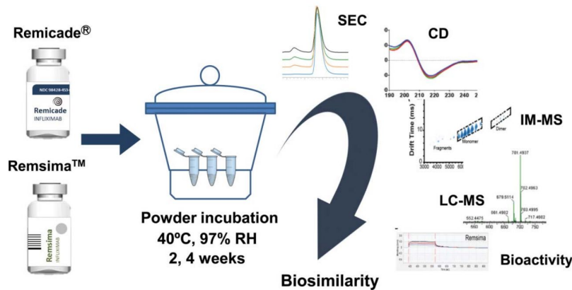
Figure 3-1. Schematic of stress study design. Humidity/thermal stress of infliximab samples were performed by incubating the drug powders at 40°C at different %RH for 0–4 weeks, followed by reconstitution (in WFI) and analysis.
