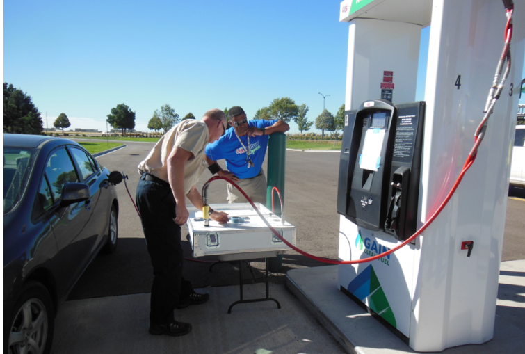
Figure 7.1. A gas dispenser's metering accuracy is tested through various Weights and Measures Programs. A photo was taken from 'Taking Measure' blog of the National Institute of Standards and Technology (NIST) (Credit: T.Butcher, NIST [1]).
