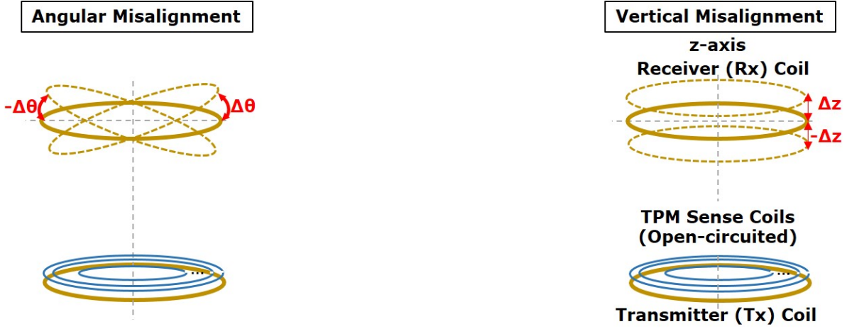
Figure 3.13. Angular misalignment (left) and vertical misalignment (right) between the Tx and Rx coils.
