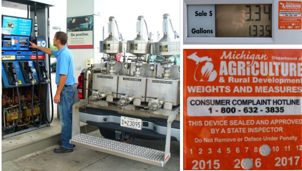
Figure 2.1. US Weights and Measure Program qualifies secured gas pump metering (left) with a seal (right). [Photo (left): Weights and Measures, Maryland Department of Agriculture]
