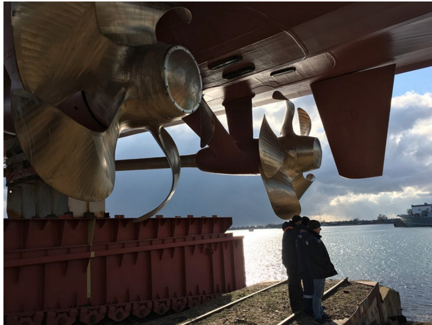
Figure 1.4: Propellers with highly skewed and curved blades 2
