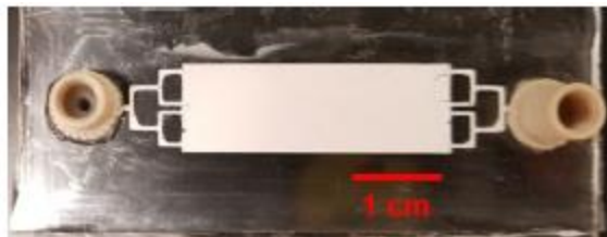
Figure 7.1: Photograph of a Nanodisc formation device fabricated using hot embossing in cyclic olefin copolymer. A C_{18} acrylate monolith was then directly photopolymerized within the device.
