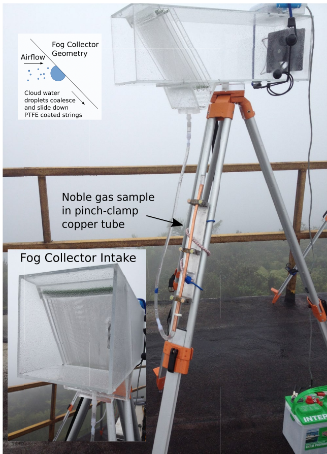
Figure 2. Battery powered fog collector set up at Pico del Este, Puerto Rico. Upper inset shows the basic geometry of the collector, where cloud water droplets impinge on PTFE coated strings. Water drops then slide down the strings to a collection basin, and thence down a plastic tube to the bottom of a copper tube equipped with stainless steel pinch-off clamps. Filling the copper tube from the bottom reduces the chances of incorporating air bubbles.
