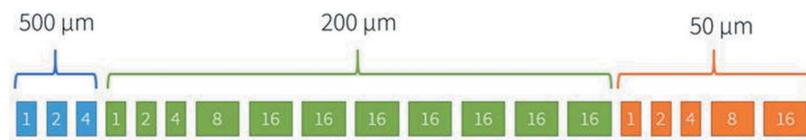
Figure 2 CRL transfocator layout at beamline 23ID-D. The numbers in the boxes show the number of lenses in each lens block and the numbers above indicate their radius of curvature. X-rays propagate from left to right.
