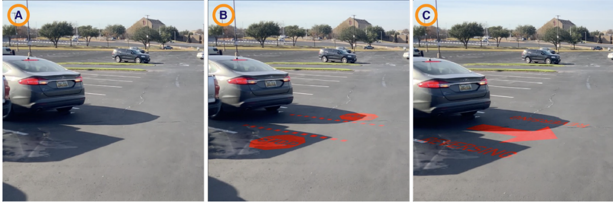
Figure 5-2: Projected Messages in Simulator Video: A) Brake Light Only, B) Stop Signs (Pedestrian Instruction), C) Reversing Arrows (Vehicle Intent)
