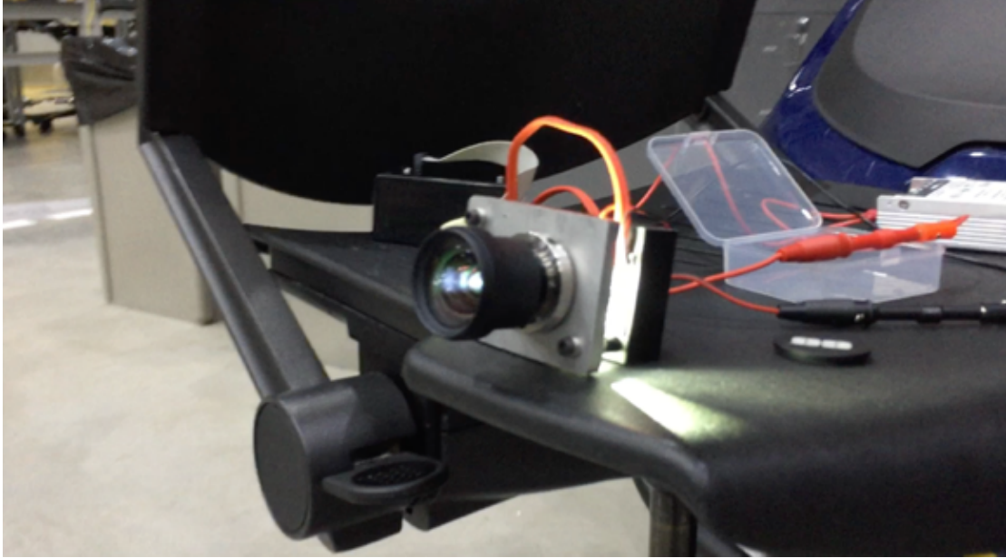
Figure 3-3: OSRAM EVIYOS Lamp set up for testing
