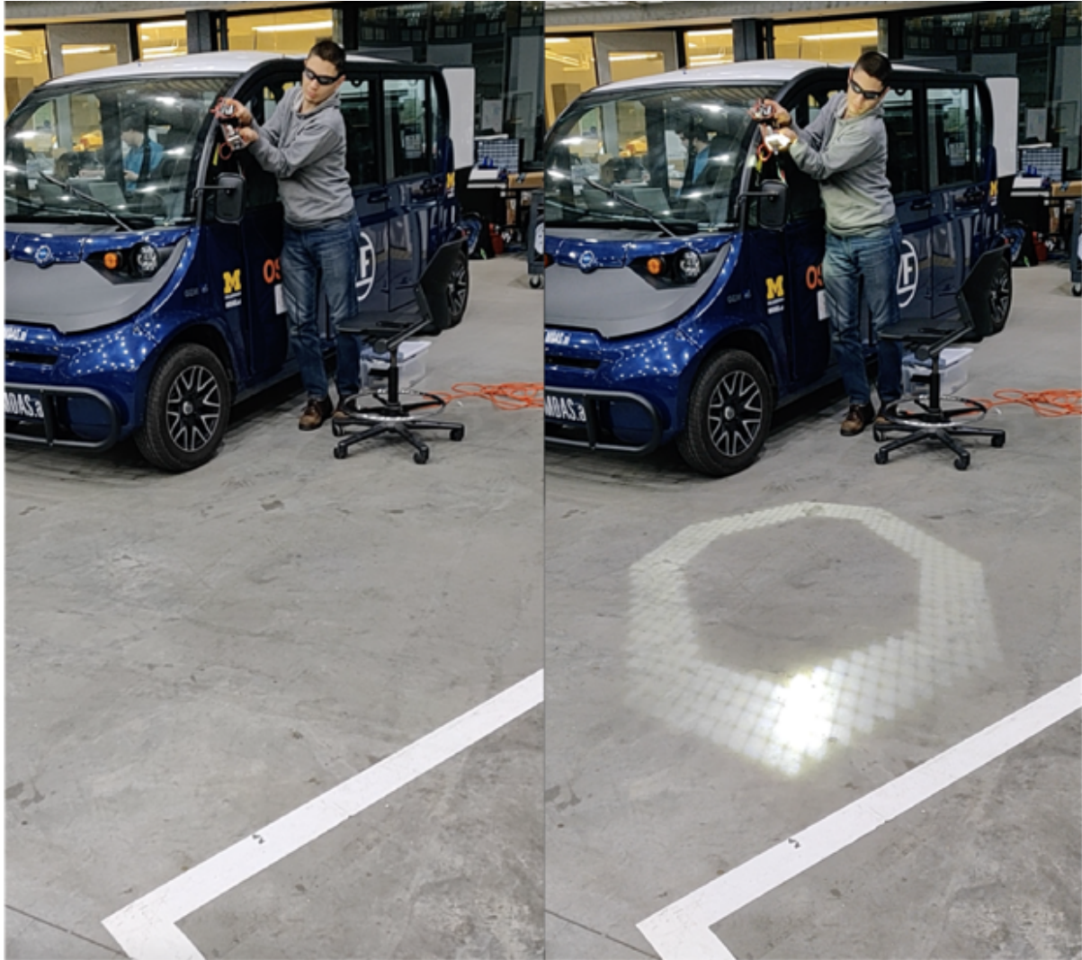
Figure 3-5: A University of Michigan student demonstrates the EVIYOS projector array from a position on the A-pillar of the MDAS.ai shuttle. An image of a white octagon is projected onto the ground in front of the shuttle.
