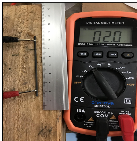
Figure 23. The setup with the graphite rod, the multimeter, and a ruler showing the length of the rod which is roughly 6 cm between the leads.
