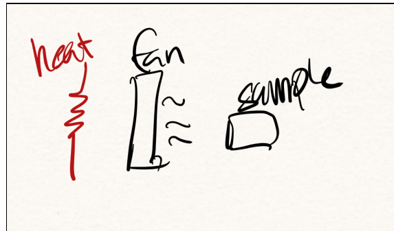
Figure A5. A second design for the “heating the sample” sub-function. This design features a fan blowing hot air onto the sample. This will decrease the amount of heat the heating element needs to put out compared to other designs, but accuracy and consistency of the heat are an issue.
