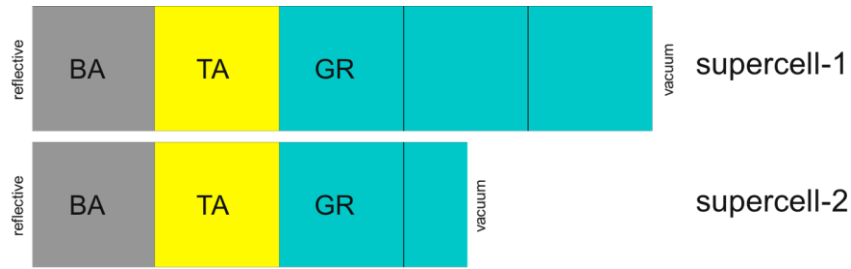
Figure 4.5 Supercell Models for Thermal Assembly in Homogenized CFTR-1D (Vacuum conditions on the right are replaced with reflective ones when albedo search is invoked.)
