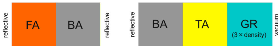
Figure 3.8 Illustration of Supercell Models for Fast (FA) and Thermal (TA) Fuel Assemblies
