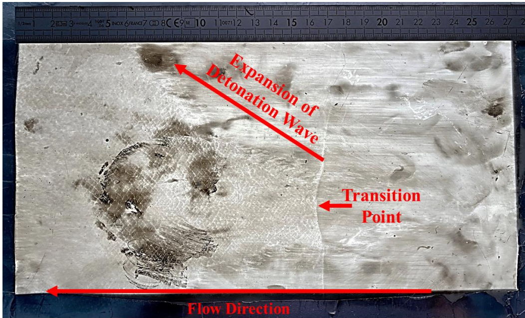
Figure 5.11: Transition to detonation captured by the soot foil showing the transition point and the expansion of the detonation wave within the tube. The change in cell size structure is also of interest, with the detonation cells expanding slightly as the wave forms due to the initially overdriven detonation wave beginning to relax to the DCJ condition.
