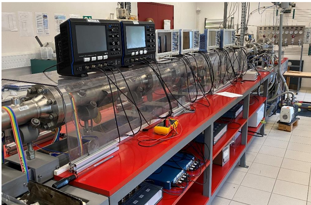
Figure 5.6: Shock tube setup at CNRS-ICARE.
