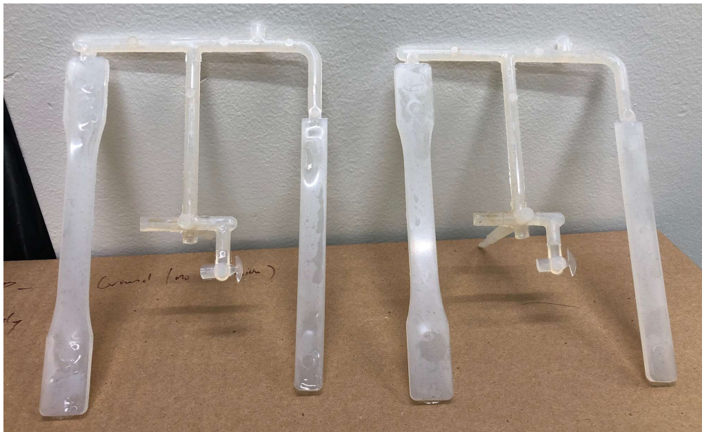
Figure 2.4. Samples with (left) and without (right) sink marks.
