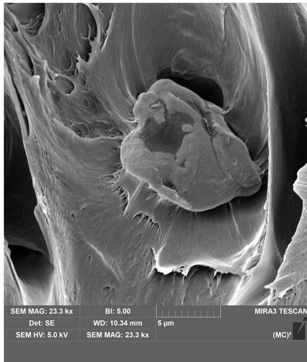
Figure 5.3. Fracture surface of 5% CNC-reinforced PA610 at magnification 23.3 x.
