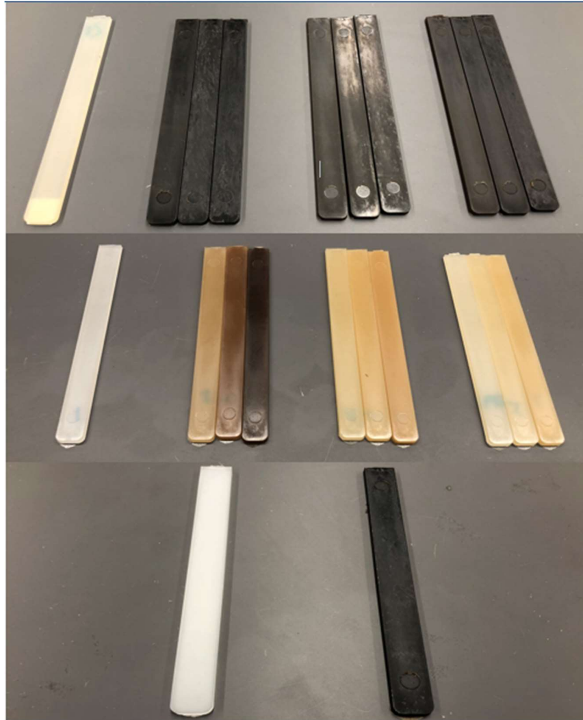
Figure 2.6. Appearance of the parts. First row, PA610: left to the right- control; 2.5%, 5%, 10% CNC filled; 2.5%, 5%, 10% 4 \mu m cellulose filled; 2.5%, 5%, 10% 100 \mu m cellulose filled. Second row, PP: left to the right- control; 2.5%, 5%, 10% CNC filled; 2.5%, 5%, 10% 4 \mu m cellulose filled; 2.5%, 5%, 10% 100 \mu m cellulose filled. Third row, PA1010: left to the right- control; 5% CNC filled.
