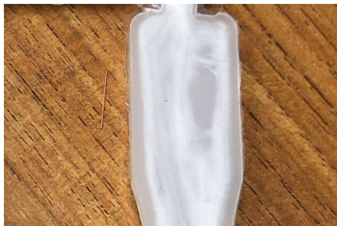
Figure 2.2. Flow lines in an injection molded part.
