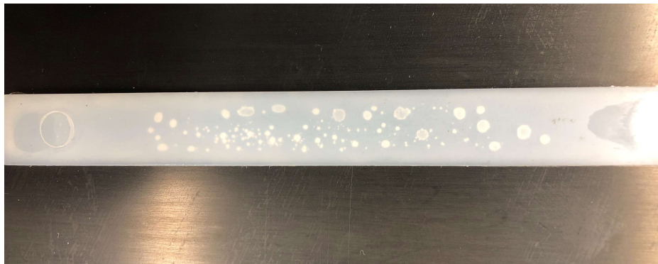
Figure 2.3. Vacuum voids in an injection molded part.
