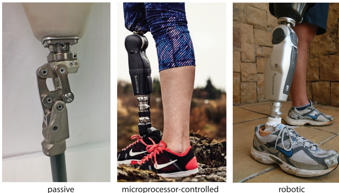
Figure 7.2: An example of each prosthesis type. Image adapted from Ossur Total Knee, Ossur Rheo Knee, and Ossur Power Knee images.
