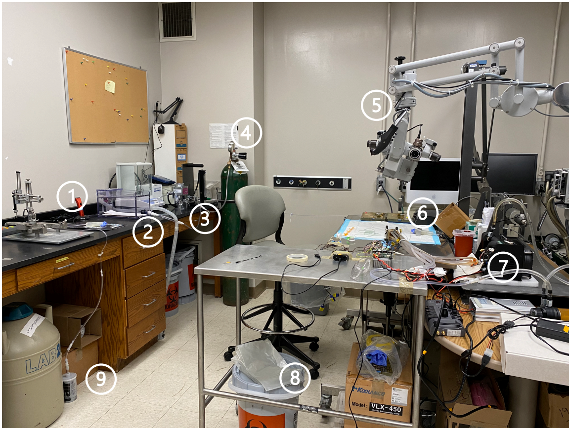
Appendix Figure 1. Rat surgical space setup. 1) Kopf stereotaxic frame, 2) anesthesia induction box and shaving area, 3) Vetamac isoflurane vaporizer, 4) oxygen tank with regulator, 5) 10x microscope, 6) surgical benchtop with anesthesia nose cone and cooling probe tip, 7) Koolance cooling probe chiller and power supply, 8) biohazardous waste disposal, 9) charcoal canister for waste isoflurane recovery, with another under the surgical benchtop.
