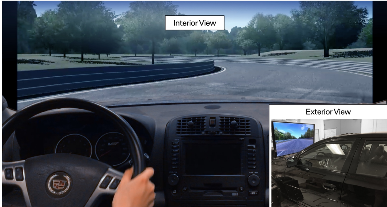
Figure 12. The driving simulator for the pneumatic steering column. From the interior of this vehicle (main), the participant used an interaction prototype that was built into the steering column to control the vehicle in the simulated environment (VI-DriveSim). This simulator was housed in a 2004 Cadillac CTS-V (exterior view; bottom right) to provide an immersive environment. The rapid-steering track is pictured here.
