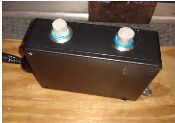
Figure 13. Controller with flush buttons modified with soft raised extensions.
