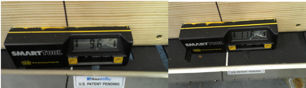
Figure 16. Demonstration of static ramp strength test procedure: applying static load through loading crate, and slope measurement before and after loading.
