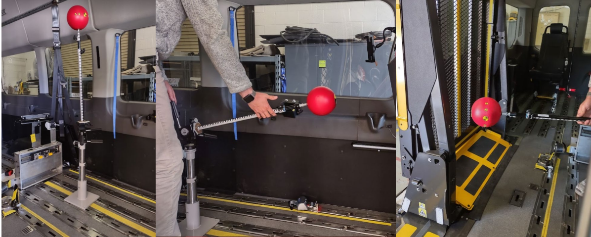
Figure 20. Photos demonstrating use of adapted tool, set to the forward-high location of the wheelchair station (left). When the upper component is adjusted to the longest setting, it would not contact the forward panel behind the driver (center) or the stowed wheelchair lift (right).
