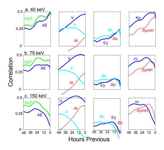
Figure 1. Cross correlations between GOES electron flux and possible drivers (hourly averages) for a. 40 keV, b. 75 keV, c. 150 keV. Solid lines are positive correlations; dashed lines are negative correlations. Note that most correlations are < 0.5 in magnitude.
