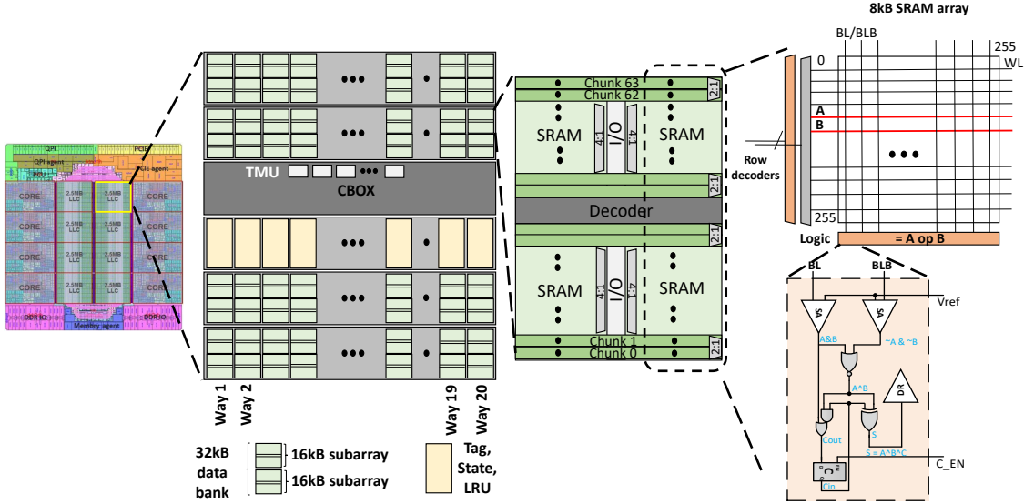
Figure 4.1: Neural Cache overview. (a) Multi-core processor with 8-24 Last Level Cache (LLC) slices. (b) Cache geometry of a single 2.5MB LLC cache slice with 80 32KB banks. Each 32KB bank has two 16KB sub-arrays. (c) One 16KB sub-array composed of two 8KB SRAM arrays. (d) One 8KB SRAM array re-purposed to store data and do bit line computation on operand stored in rows (A and B), (e) Peripherals of the SRAM array to support computation.
