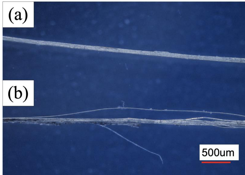
Figure 2.15 Optical microscopy for (a) lab scale enzyme retted stem fibers (b) dew retted stem fibers
