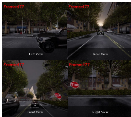
Figure 5-3 360-degree perception coverage around the ego vehicle using four RGB cameras.
