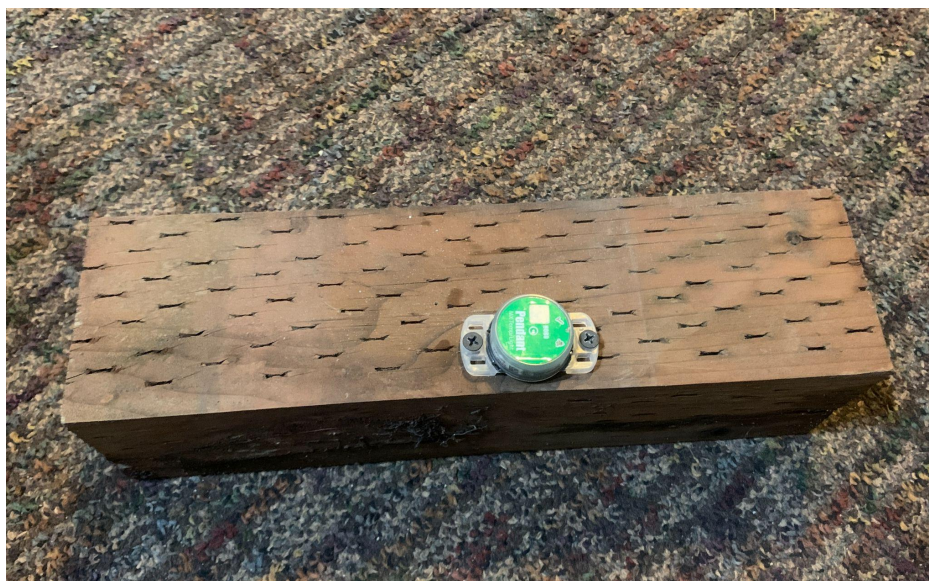
Figure 15. The data logger was screwed onto a wooden block.
