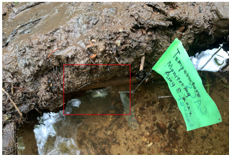
Figure 16. An illustration of the data logger and how the wooden block is stabilized by a heavy branch and the mud.
