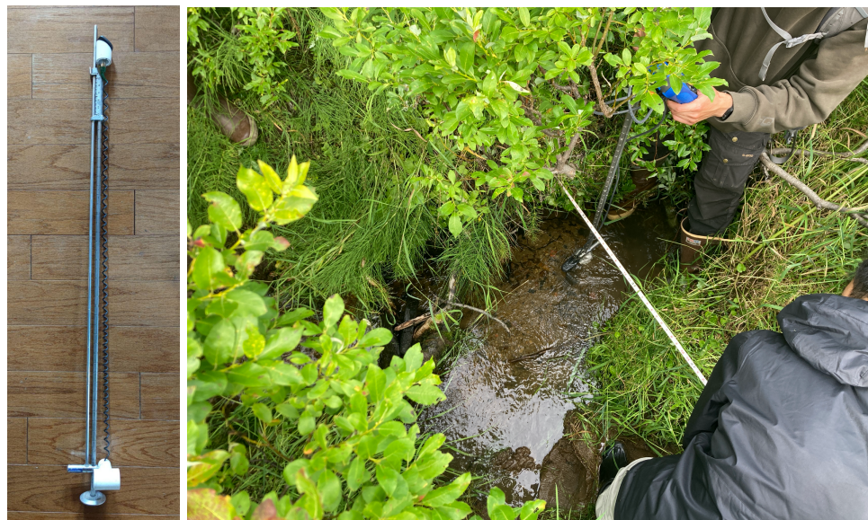
Figure 9. The Turbo-Prop flow meter (left) utilized to measure water velocity (right).
