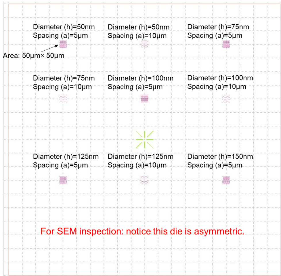
Figure 6.4: Schematic of 50 μm x 50 μm dice with different diameters and spacings. The die is asymmetric, which was used for SEM inspection of the pattern.
