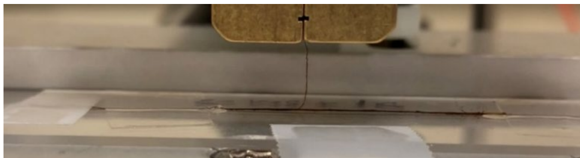
Figure 2.7: Peel test performed on technical flax fibers. A small portion of fiber was peeled away from the remaining technical fiber and the maximum force was recorded. Values were subsequently normalized to the peel diameter.
