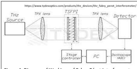
Figure 1: Diagram of Workings of Fabry-Pérot Interferometer
