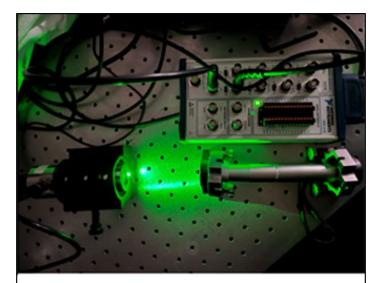
*Figure 2:* Experimental Setup; FPI receives light source and sends data to the PC to be processed
