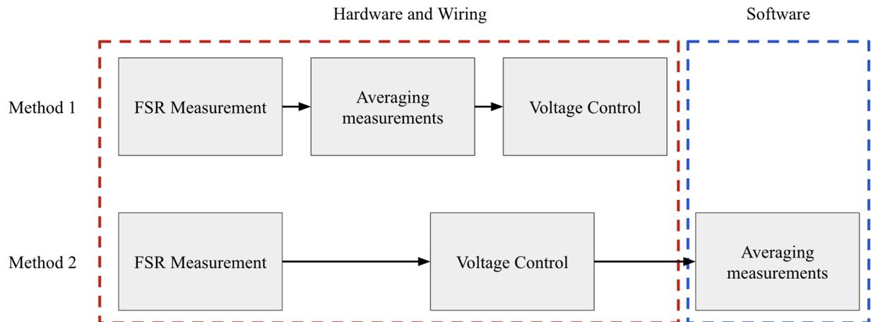
**Figure 9:** Differences between the two wiring systems. Blocks represent data and conversions.
