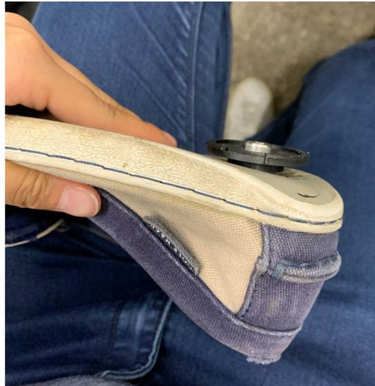
**Figure 3:** Validating the screw-in securement method with an initial design of the protective cover's base.
