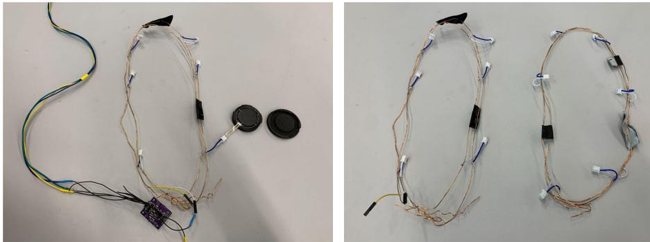
**Figure 6:** The electrical wiring system, without the shoes. The oblong shapes are the two copper parallels. Soldered around each edge are inserts for each sensor.
