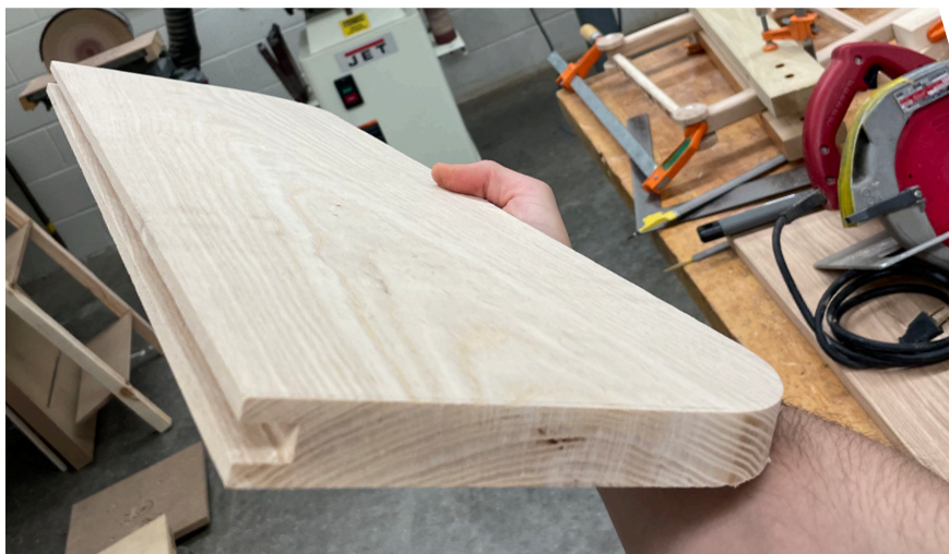
21 BRIDLE GROOVE CUT INTO A TABLETOP ENDCAP
