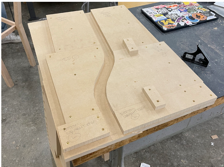
10 A TWO-PART MDF BENDING FORM
