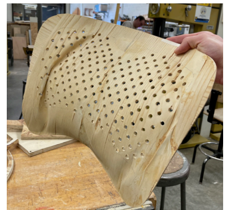
28 DRILLING HOLES IN THE BACKREST, WRINKLE VISIBLE AT LEFT
