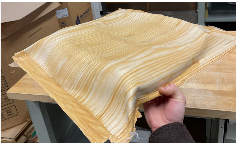
25 VACUUM PRESSED LAMINATION BEFORE BEING TRIMMED
