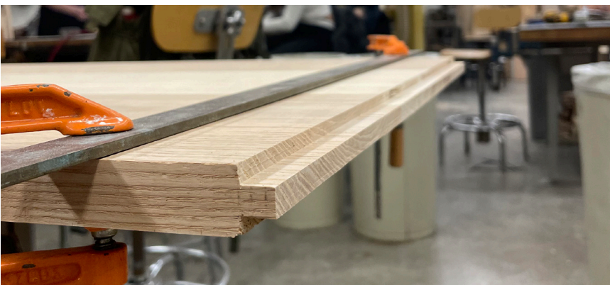
20 ROUTED TENON ON A SOLID TABLETOP
