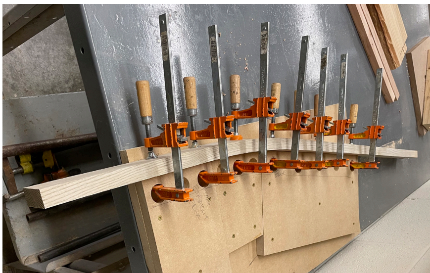
6 BENDING A TEST PIECE ON AN MDF BENDING FORM
