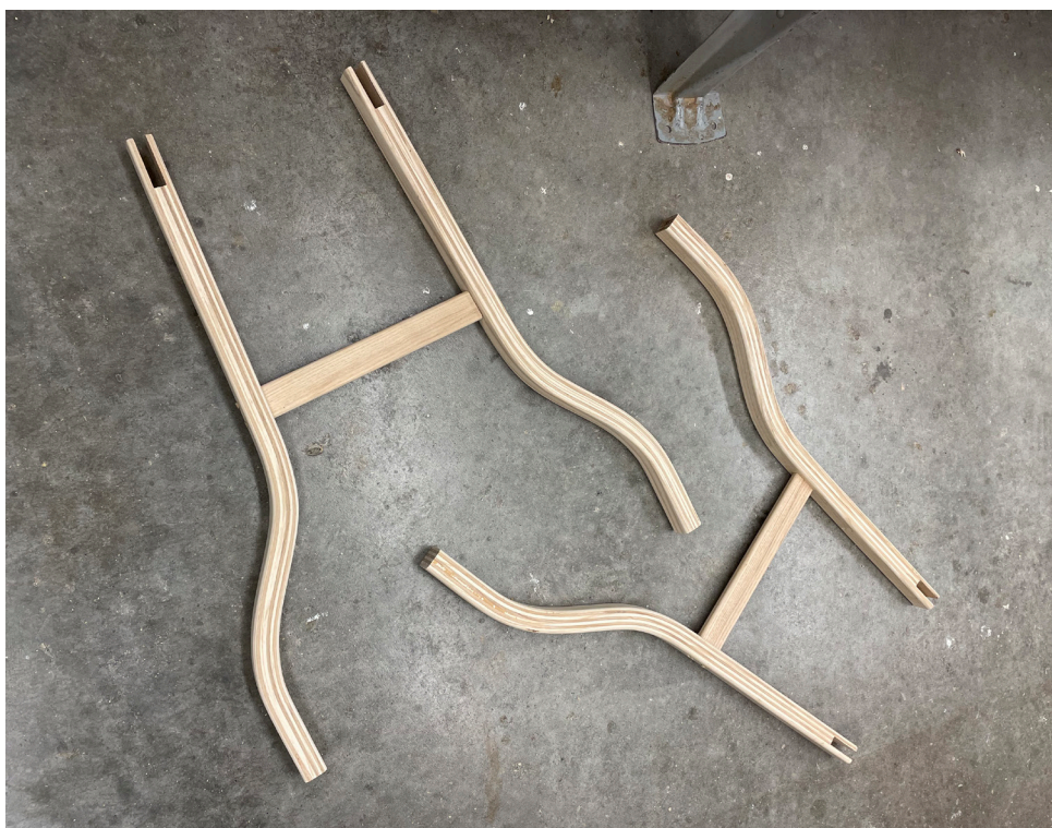
23 TEST FITTING TWO TABLE FRAMES WITH THEIR STRETCHERS
