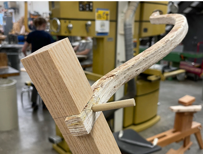
19 TEST FITTING AN OSB STRETCHER INTO A HALF-LAP JOINT
