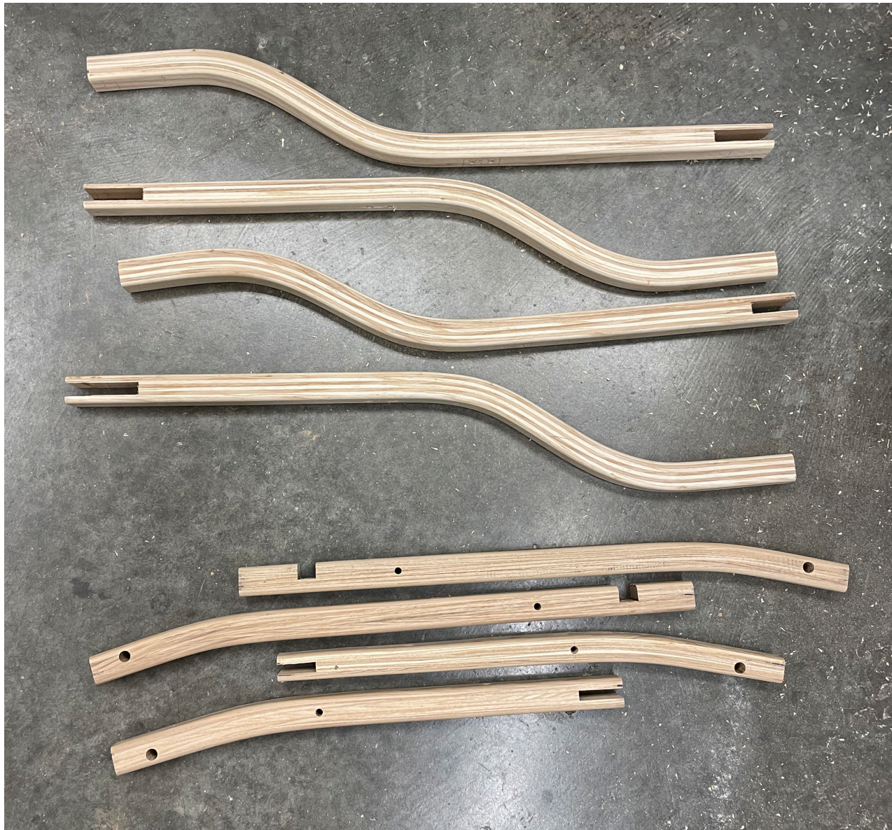
16 FINISHED STRIP LAMINATED PIECES
