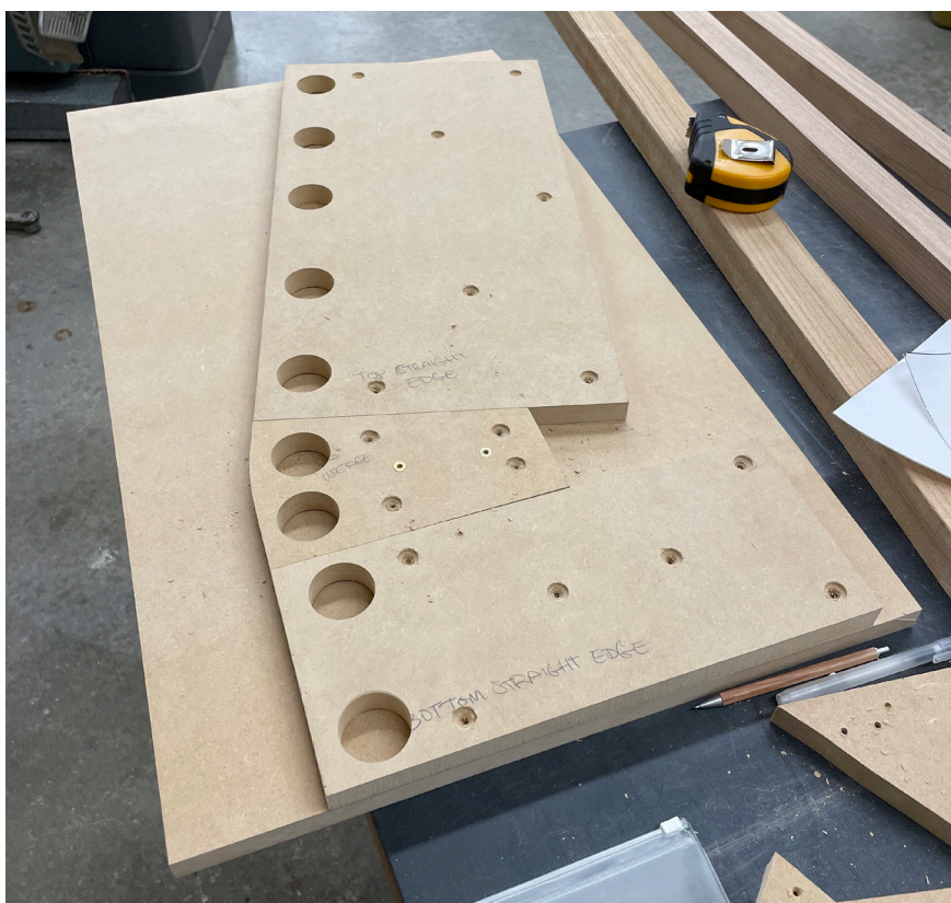
11 A ONE-PART MDF BENDING FORM
