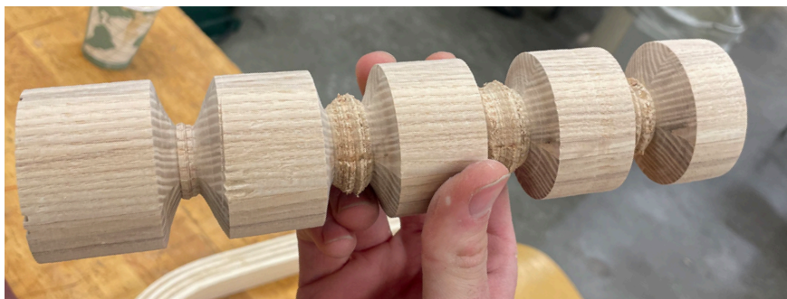
22 TURNED BEADS BEFORE BEING CUT INTO CASTERS
