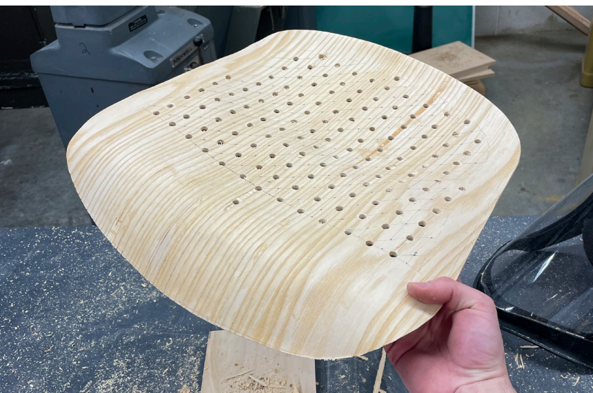
26 DRILLING HOLES IN THE TRIMMED FORM
