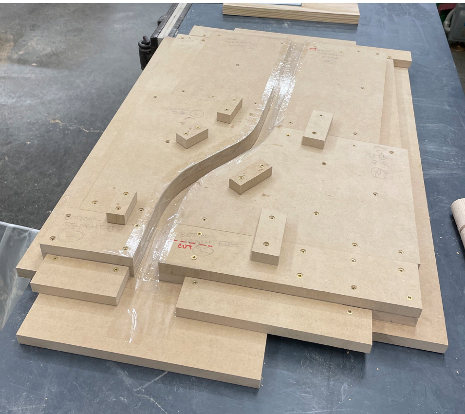
13 A MODIFIED TWO-PART BENDING FORM
