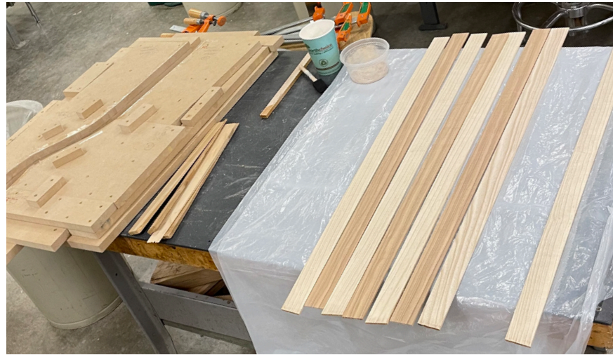
15 PREPARATION OF STRIPS BEFORE GLUE-UP
