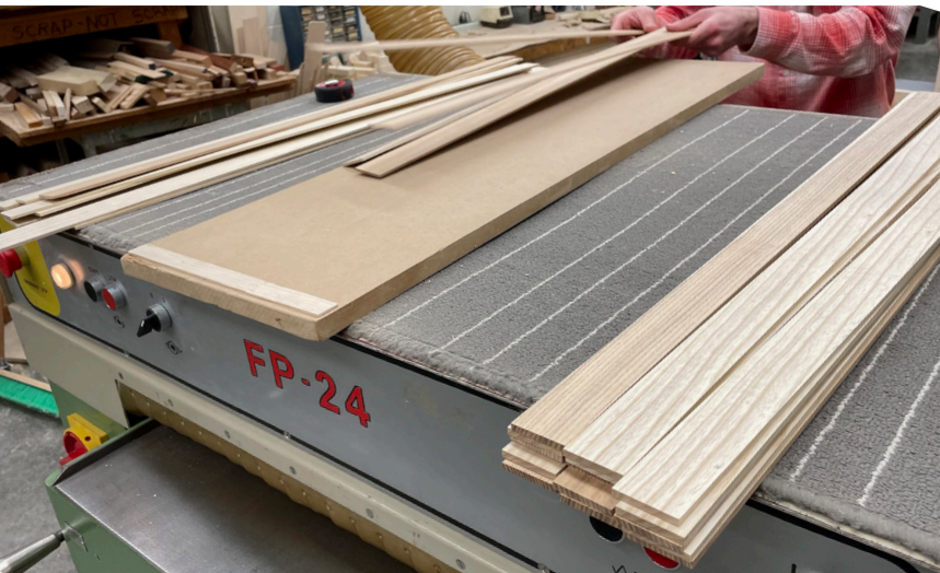
9 STRIPS BEING PASSED THROUGH THE PLANER ON AN MDF SLED
