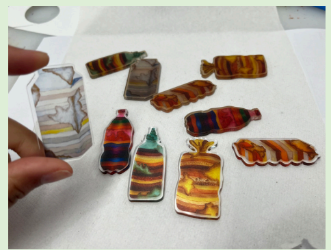
Using laser cutter on acrylic to cut shapes and UV printer to print mini version of woodpanel paintings.
