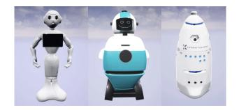
**Figure 2.** Three Security Robots: Pepper (Left), RAMSEE (Middle), and Knightscope K5 (Right)
