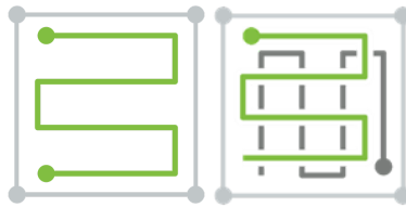
Figure 2. Depiction of a single and double grid flight plane (PIX4D, 2019).
