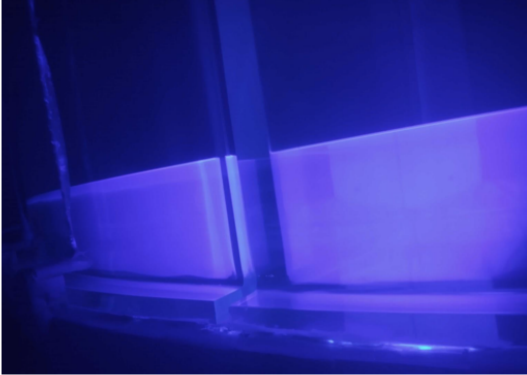
Figure 2.16: UV photograph of the bottom acrylic vessels filled with a few centimeters of Gd-LS.
