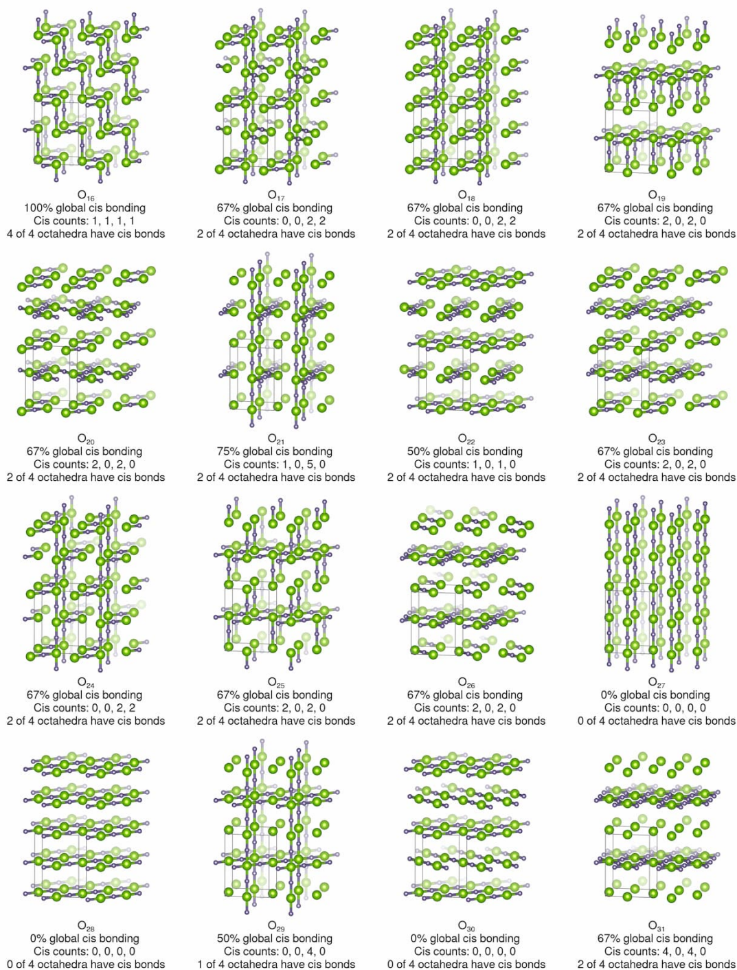
Figure C.5: ( continued ) 2 \times 2 \times 4 PON supercells showing bonds between the B-site cations (green) and the M-site minority-composition anions (dark gray). The label under each atom rendering quantifies the cis bonding for that anion ordering. The “global cis bonding” value is the fraction of cis M–B–M bonds relative to the total number of octahedron-specific M–B–M bonds that exist within the entire supercell. The “Cis counts” values indicate how many cis bonds are detected in each octahedron, counted as shown in Figure C.4(c) , with the octahedra in no particular order. The last line shows how many of the four octahedra contain at least one cis bond. For simplicity, ideal (unrelaxed) geometries are shown.
