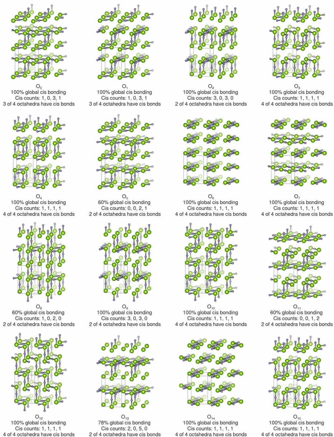
Figure C.5: 2 \times 2 \times 4 PON supercells showing bonds between the B-site cations (green) and the M-site minority-composition anions (dark gray). The label under each atom rendering quantifies the cis bonding for that anion ordering. The “global cis bonding” value is the fraction of cis M–B–M bonds relative to the total number of octahedron-specific M–B–M bonds that exist within the entire supercell. The “Cis counts” values indicate how many cis bonds are detected in each octahedron, counted as shown in Figure C.4(c) , with the octahedra in no particular order. The last line shows how many of the four octahedra contain at least one cis bond. For simplicity, ideal (unrelaxed) geometries are shown.
