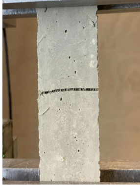
Figure 3-21. Representative crack patterns for OPC-0S20, 0% WPE and 2% sisal fiber, ECC under ultimate tensile strain.
