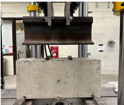
Figure 2-35. Test setup for deep beam and the multiple cracks formation at failure
