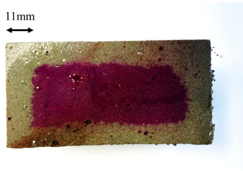
Figure 2-6 Carbonation depth of ECC beam specimen.
