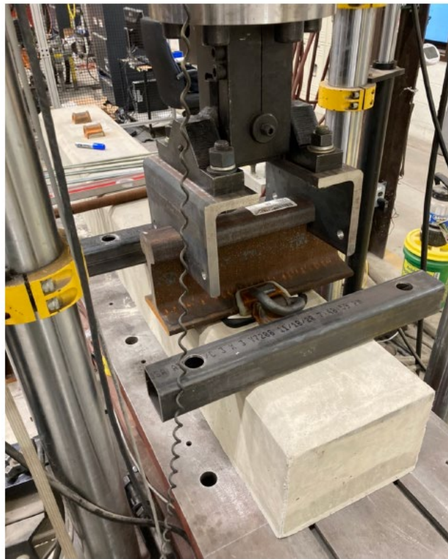
Figure 2-29. Test 5A setup for fastener uplift test
