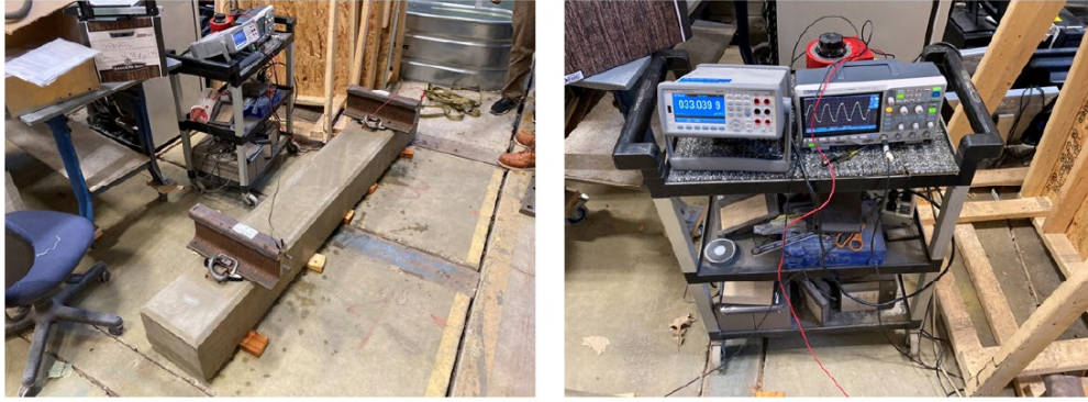
Figure 2-30. Test 7A setup for impedance test
