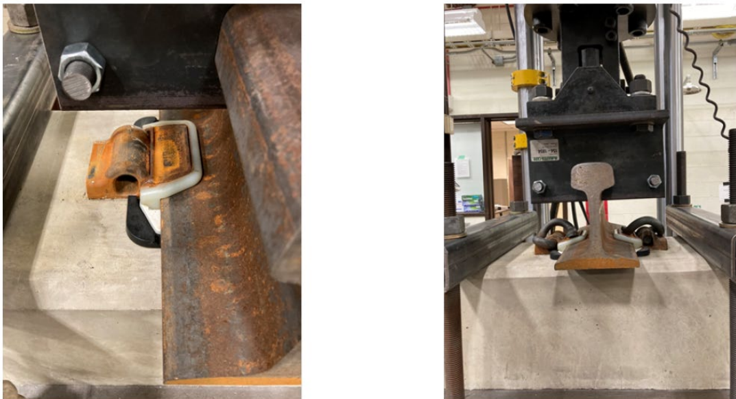
Figure 2-31. Post-test condition for fastener system
