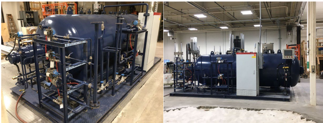
Figure 2-20. Large-scale reactor for carbonation curing.
