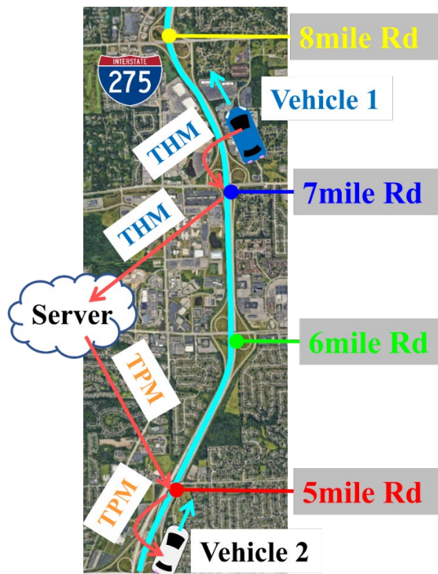
Figure 11: Experimental setup for testing CV2X infrastructure. Two connected vehicles equipped with OBUs, four RSUs, and a U of M server were used in the experiments.
