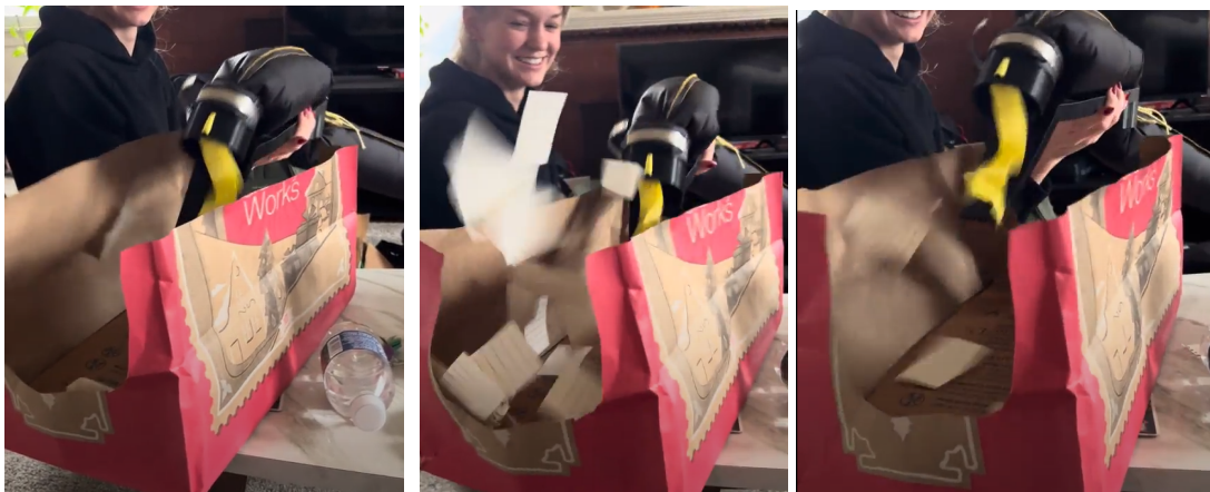
Images 9.2 - 9.4. Clips of the testing of the ripstop continuation prototype. Image 9.2 shows the gutter viper when the leaf blower had just been turned on. Image 9.3 shows the “leaves” being
