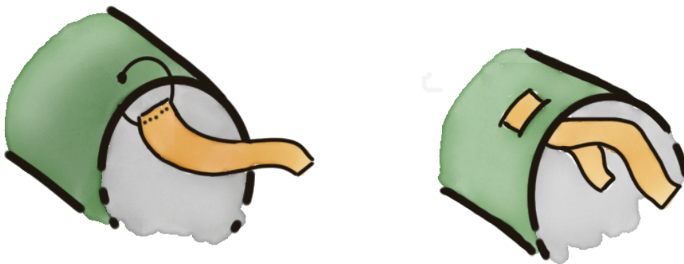
Figure 6.5: Keychain tongue assembly method (left) vs backpack strap friction tongue assembly method (right).
