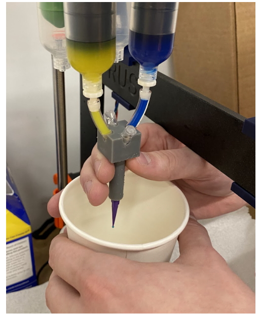
Figure 24c. Verification test 2A. The two silicone parts of EcoFlex 00-50 are extruded with equal volume and flow rates. The materials are mixed to form a green color as seen at the end of the nozzle
