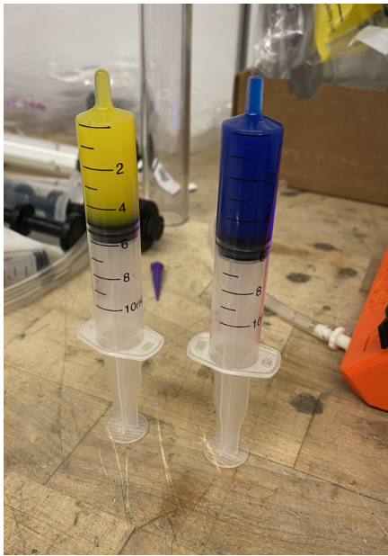
Figure 24a. Syringes used to measure equal parts of EcoFlex 00-50 Part A (yellow) and Part B (blue).
