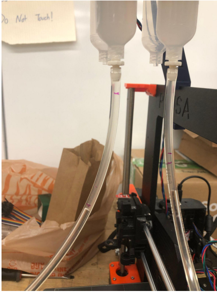
Figure 26a. Picture of experimental setup used to measure output of motor-syringe system
