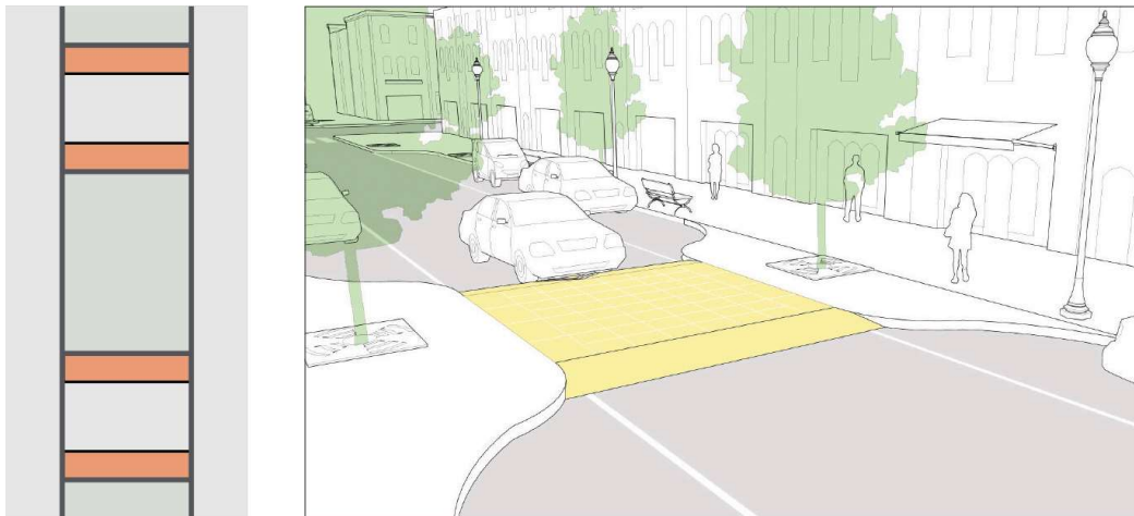
Figure 14. NACTO Concept that illustrates speed tables along roadways [16]
