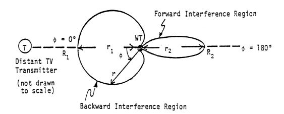
Fig. 2: Sketch of the TV Interference Zone of a WT.
