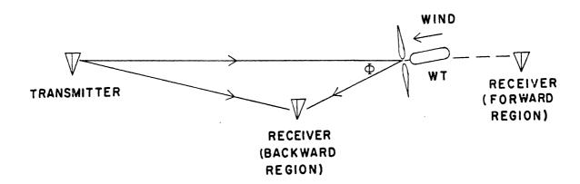
Fig. 1: Geometry of the WT Blade Scattering.
