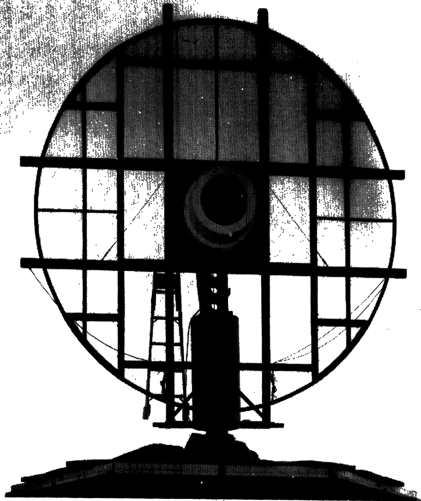
FIG. 5: Photograph of the Double Alford Loop Above the 15' Diameter Counterpoise.
