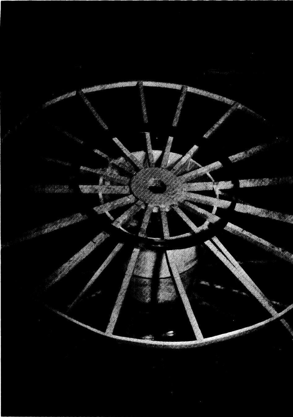
FIG. 3-7: PHOTOGRAPH OF THE PARASITIC LOOP COUNTERPOISE ANTENNA.
