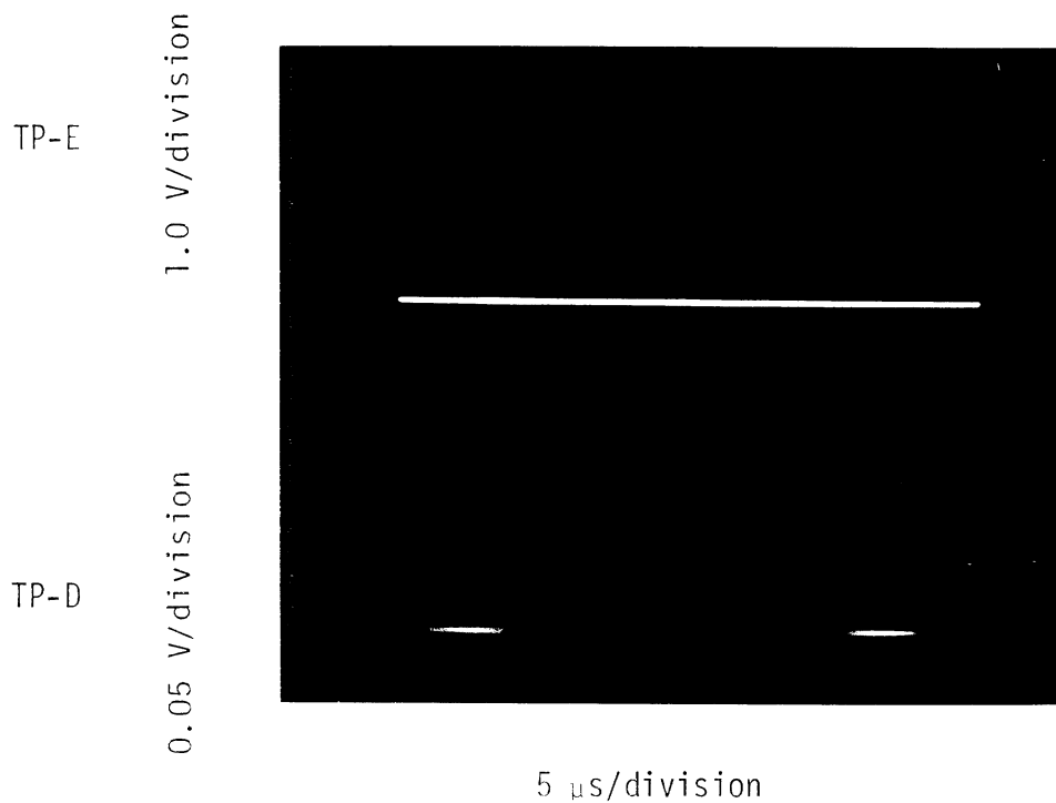
Figure 26. Signals at test points E and D with short pulse plus RF carrier input. RF carrier amplitude = 50,000 \mu V.
