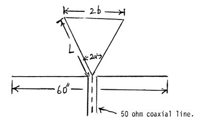
Figure 2.1 A sketch of the standard antenna.
