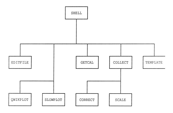
Figure 3.2 Software configuration.
