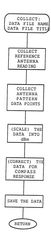
Figure 3.5 COLLECT logical flow.
