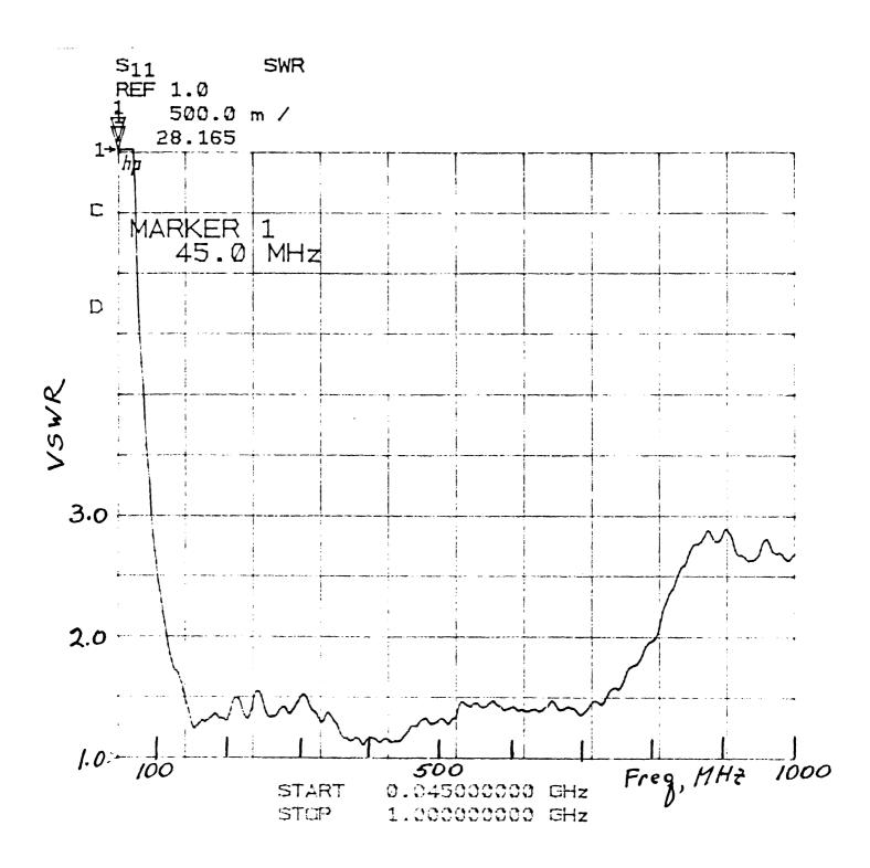
Figure 2.4 Measured VSWR characteristics of the standard antenna (Band 2: without extensions).
